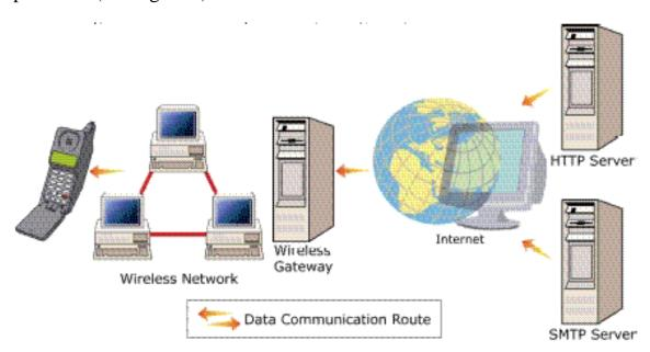
Figure 2[14]. The content threat to the wireless infrastructure involves email messages or spam that flow from SMTP or HTTP servers through wireless gateways to wireless devices.
